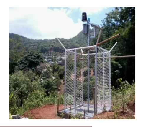
Issue: site failure detection, landslide predicting and warning system
